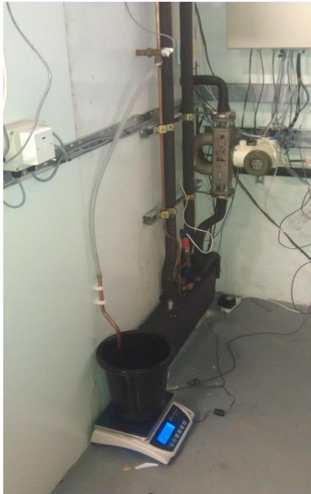
Figure 5. Insulated heat store module on floor next to cold room, Coriolis flow meter, connecting pipes and valves and digital scales for measuring melt water.
