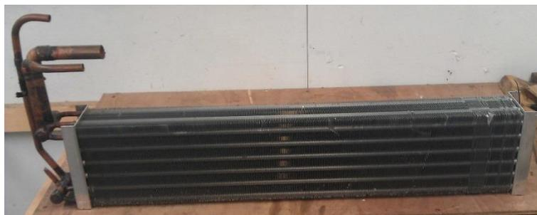
Figure 2. The finned tube heat exchanger used in the heat store module, inlet and outlet headers on the left.
